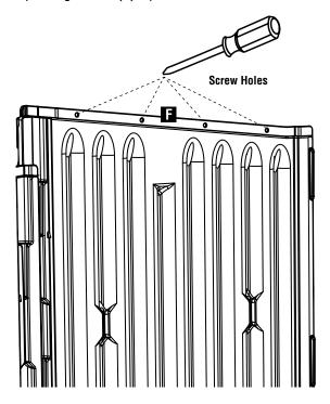
**b.** Connect **Right Back (F)** onto dovetails of **Repeat Right Side (E)**.
